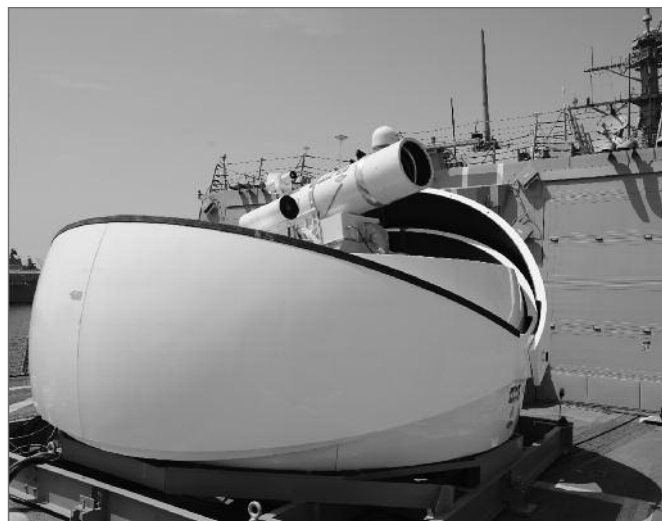
The Laser Weapon System (LaWS) temporarily installed aboard the guided-missile destroyer USS Dewey (DDG 105) in San Diego, CA is a technology demonstrator built from commercial fiber solid-state lasers. LaWS can be directed onto targets from the radar track obtained from a MK 15 Phalanx Close-In Weapon system or other targeting source.
