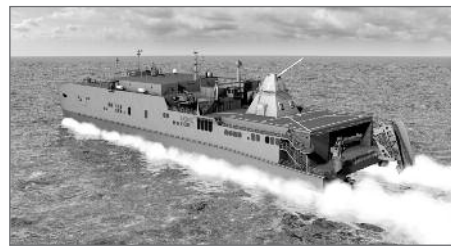
An artist rendering shows the electromagnetic railgun installed aboard the joint high-speed vessel USNS Millinocket (JHSV 3). The railgun is a long-range weapon that launches projectiles using electricity instead of chemical propellants and is currently undergoing testing at Naval Sea Systems Command, Dahlgren Division. (U.S. Navy photo illustration/Released)
