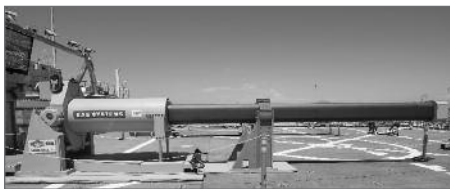
One of two electromagnetic railgun prototypes on display aboard the joint high speed vessel USS Millinocket (JHSV 3) in port at Naval Base San Diego. (U.S. Navy photo by Mass Communication Specialist 2nd Class Kristopher Kirsop/Released)
