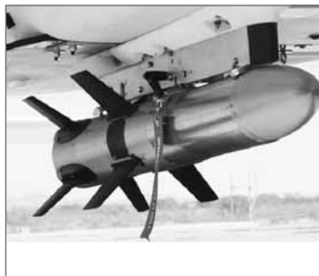
Pyros has three fusing options - height of burst, time delay and impact.
