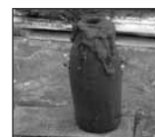
Figure 5 – The M795 after the slow cook-off test
