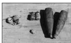
Figure 7 - Shell bodies and separated M783 fuzes from M768 cartridges recovered from the vehicle after the fire.
