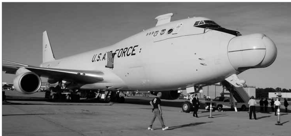
A modified 747 aircraft serves as the prototype Airborne Laser, slated to become an integral part of the U.S. missile defense system.
