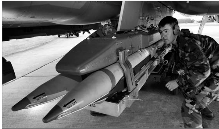
Staff Sgt. Randy Broome signals a jammer operator to move a Bomb Rack Unit 61/A forward, while loading it onto an F-15E Strike Eagle at RAF Lakenheath, England.
