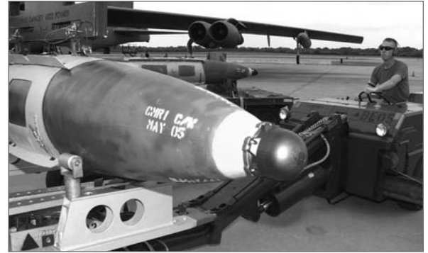
Airman 1 st Class Marcus Thames moves a JDAM that will be loaded on a B-52 Stratofortress. He is a weapons loader with the 40 th Expeditionary Maintenance Squadron at a forward-deployed location and is from Minot Air Force Base, ND
