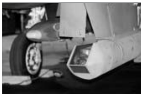
A 494th Fighter Squadron F-15E Strike Eagle equipped with the new Sniper Advanced Targeting Pod
