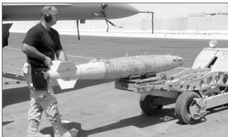
Unloading a GBU-38 from an F-16 at a forward-deployed location.
